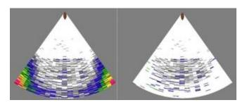
Figure 2: On left: Simrad ME70 data with TVG-enhanced noise, particularly in the outer beams; on right: the same area after applying the Background Noise Removal operator
