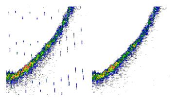
Figure 1: On left: original data with impulse noise; on right: the same area after applying the new Impulse Noise Removal operator
