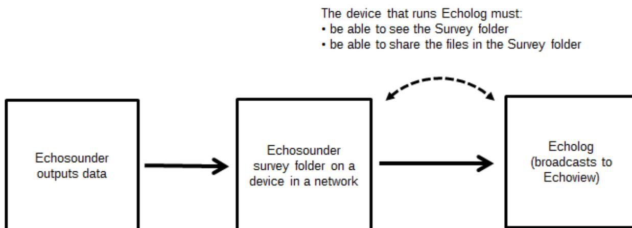
Figure 1. Flow of data under live viewing
