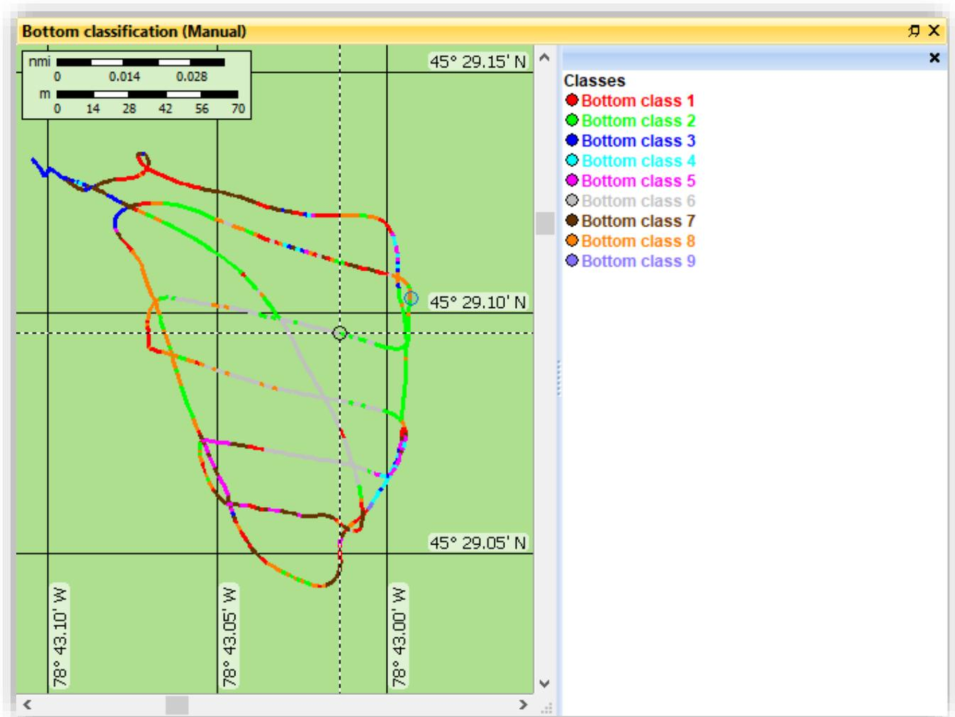
Figure 5. Bottom classification displayed as a cruise track.
