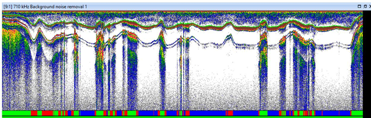
Figure 4. Echogram with bottom classification result integram shown along the bottom.
