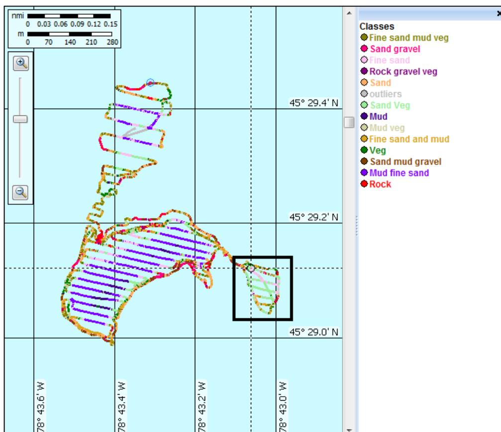
Figure 2. Cruise track showing bottom classification results of the entire survey.
